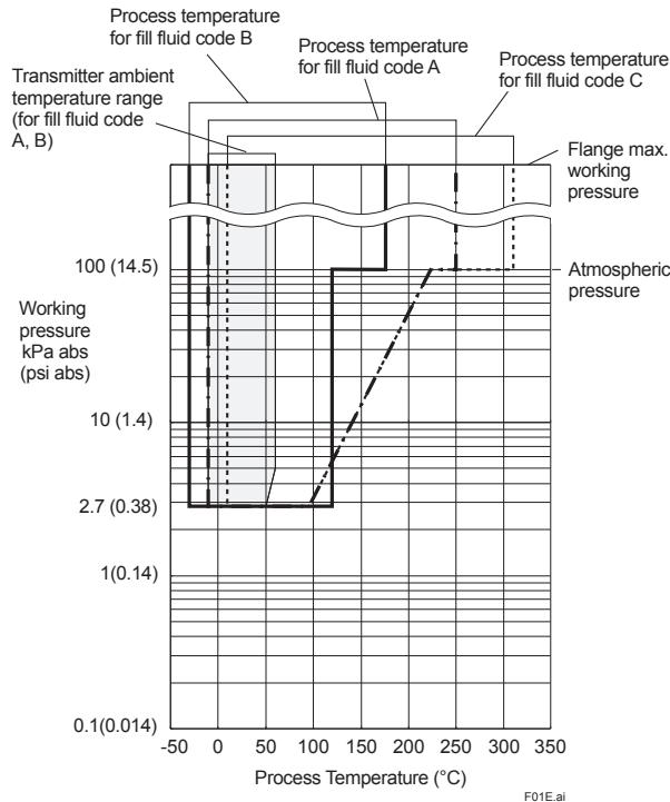
**Figure 1-1. Working Pressure and Process Temperature (Fill fluid : silicone oil for general and high temperature use)**
